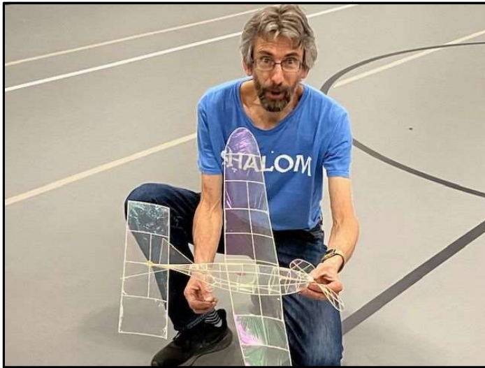
David was tickled by his Indoor ROG Cabin model, as it was using a wing that could also be shared by an Indoor Stick model. This plane flew so slowly that he was able to identify (in flight) one particular segment of a spar that was a bending a little too much under compression.
